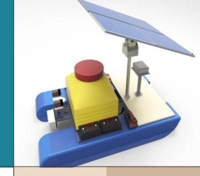
1. Intelligent and adjustable blade system with a special angle for food distribution 2. Control system and programmed board for 12-volt power consumption and boat control system 3. Designing a special body for placing equipment with the same balance on water
